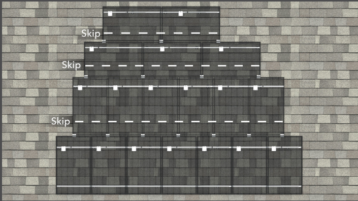
Example of Comp Roof Array
