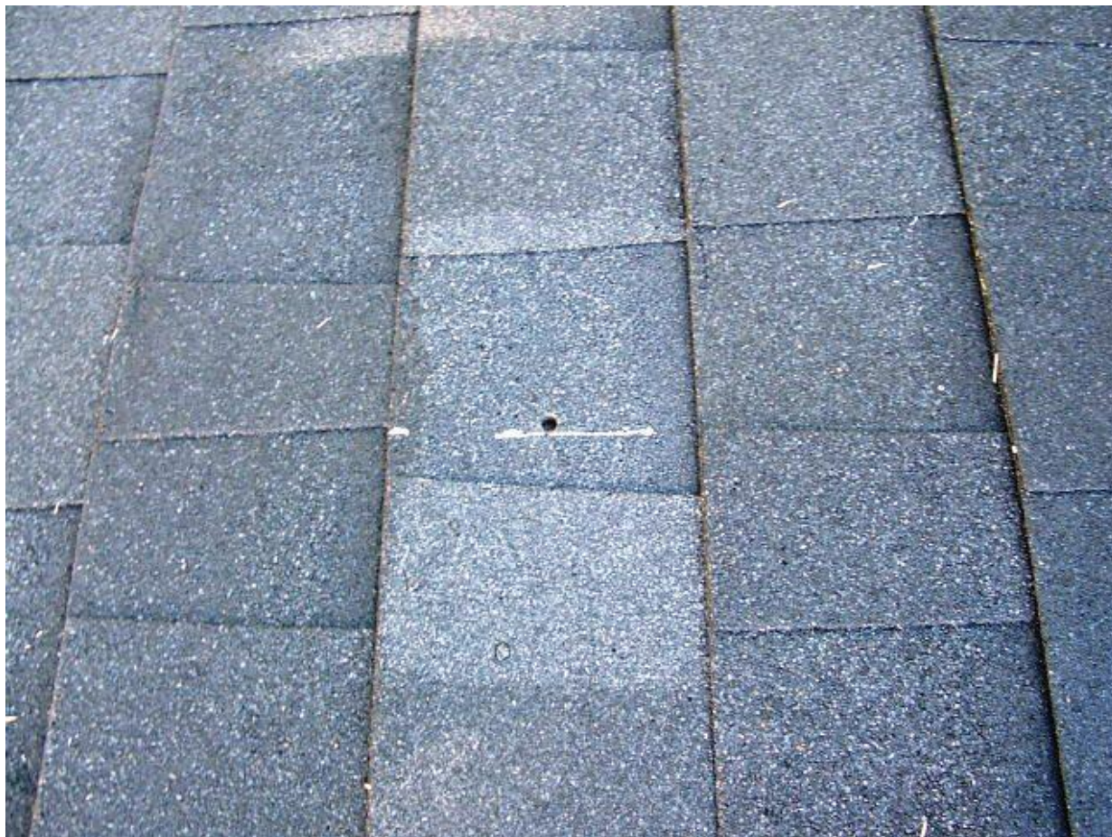
Photograph No.3 Rain Test Results No Water Penetration through or Around Roof Flashing
