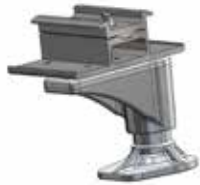
Single Mount UL 2703 Tested & Certified Tighten to 135 in-lbs
