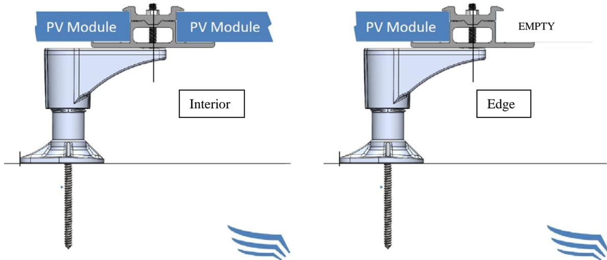
Diagram RE1. Standard Interior has PV Modules on Both Sides, Standard Edge has PV Module on One Side Only.
