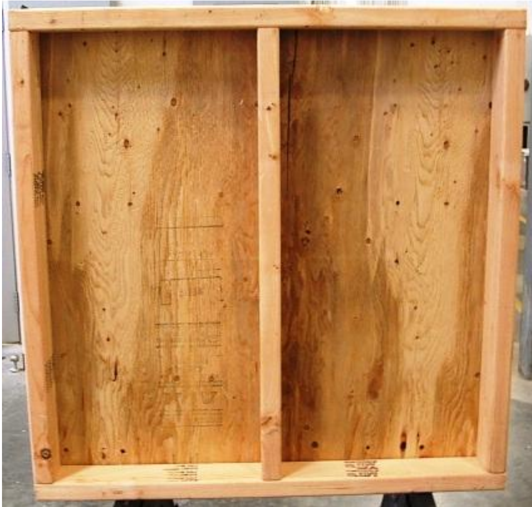
Photograph No.6 Results of Rain Test Conducted on Deck No.1 (2:12 Slope) No Water Penetration to the Underside of the Roof Deck Occurred.
