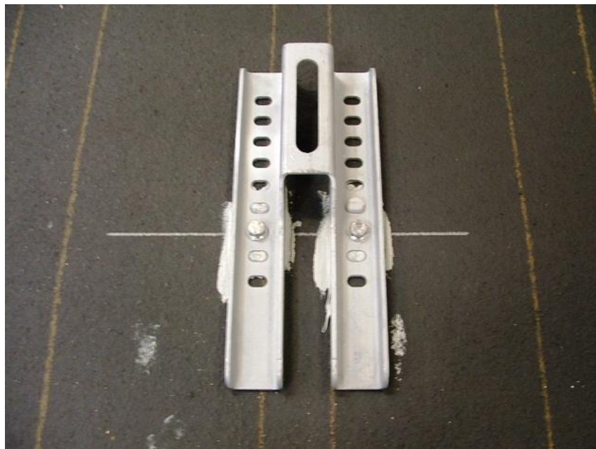
Photograph No.2 Tile Sled Mounted on Roof Deck No.2
