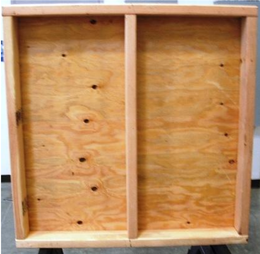
Photograph No.7 Results of Rain Test Conducted on Deck No.2 (9:12 Slope) No Water Penetration to the Underside of the Roof Deck Occurred.
